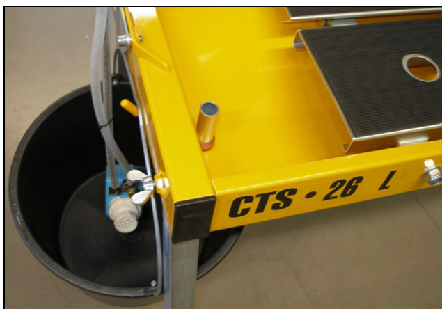
Fig. 3.17 Immersion pump in the water container, overflow pipe inserted
