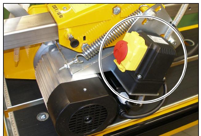
Fig. 3.15 Main switch with emergency-stop button
