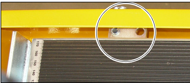
Fig. 3.5 Work table receiving on the frame
