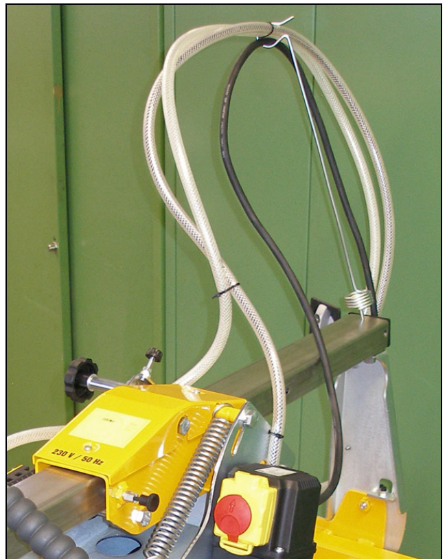
Fig. 3.8 Cable- hose holder inserted, cable- and water hose attached
