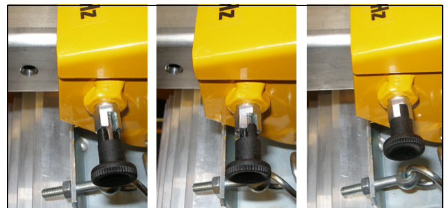
Fig. 3.11 Position of detent pin: out of function, snap position, locked into place
