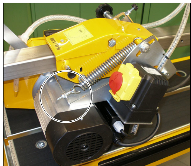
Bild. 5.24 Adjustment possibilities of the swivel cutting head compensation spring
